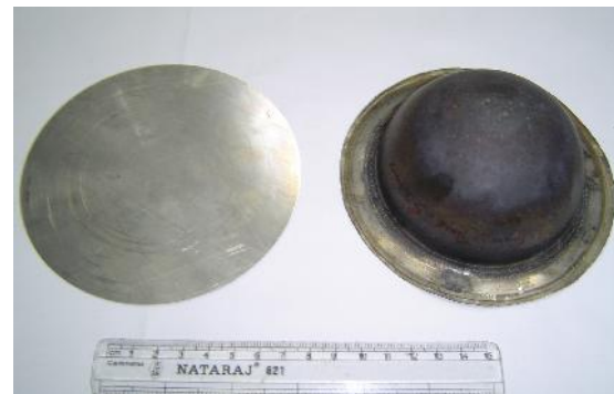
Fig.4 SPF component (right) and the blank (left) before forming.
