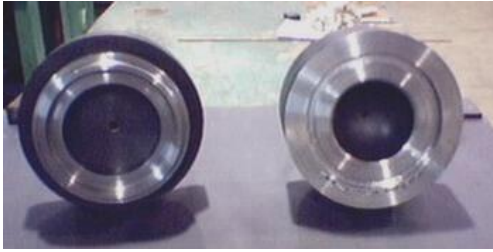
Fig.2 A picture of the top (left) and bottom (right) die for SPF.
